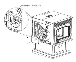
Figure 25 Exhaust blower cleaning
